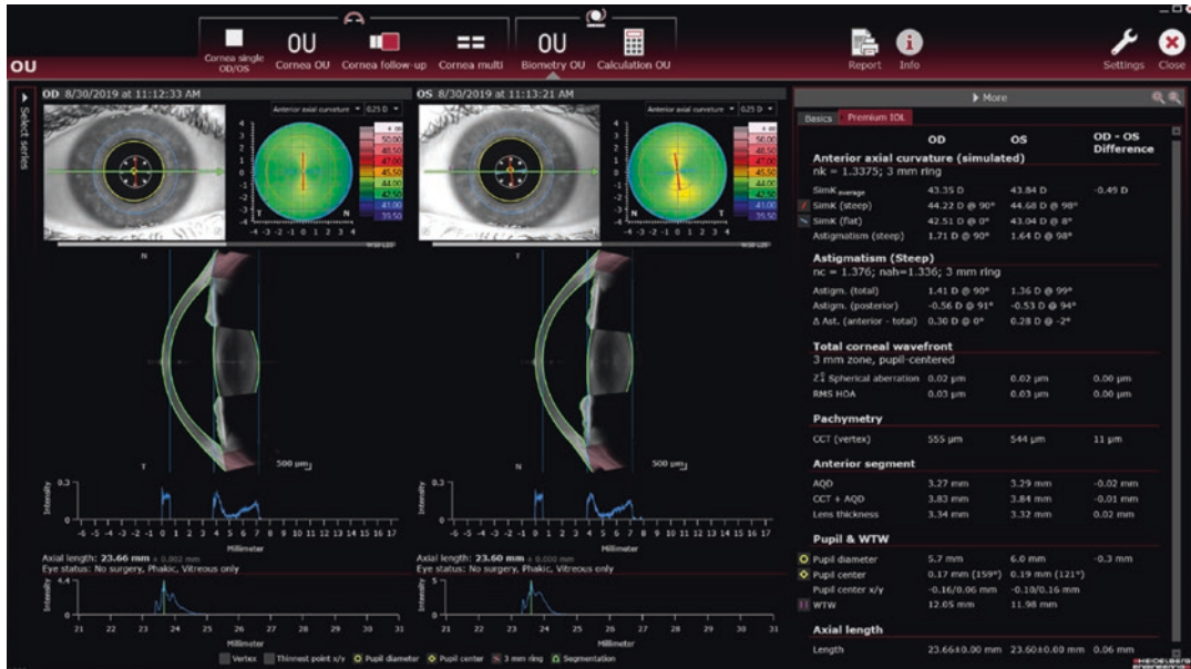
Fig. 22.4 ANTERION Cataract App: Both eyes (OU) view showing anterior axial curvature maps, OCT section images and intensity graphs, axial length diagrams, and parameters for cataract surgery planning
