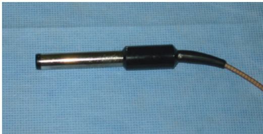
Fig. 16.5 The Kretztechnik 7200 solid probe is used for diagnostic standardized A-scanning and for biometry
